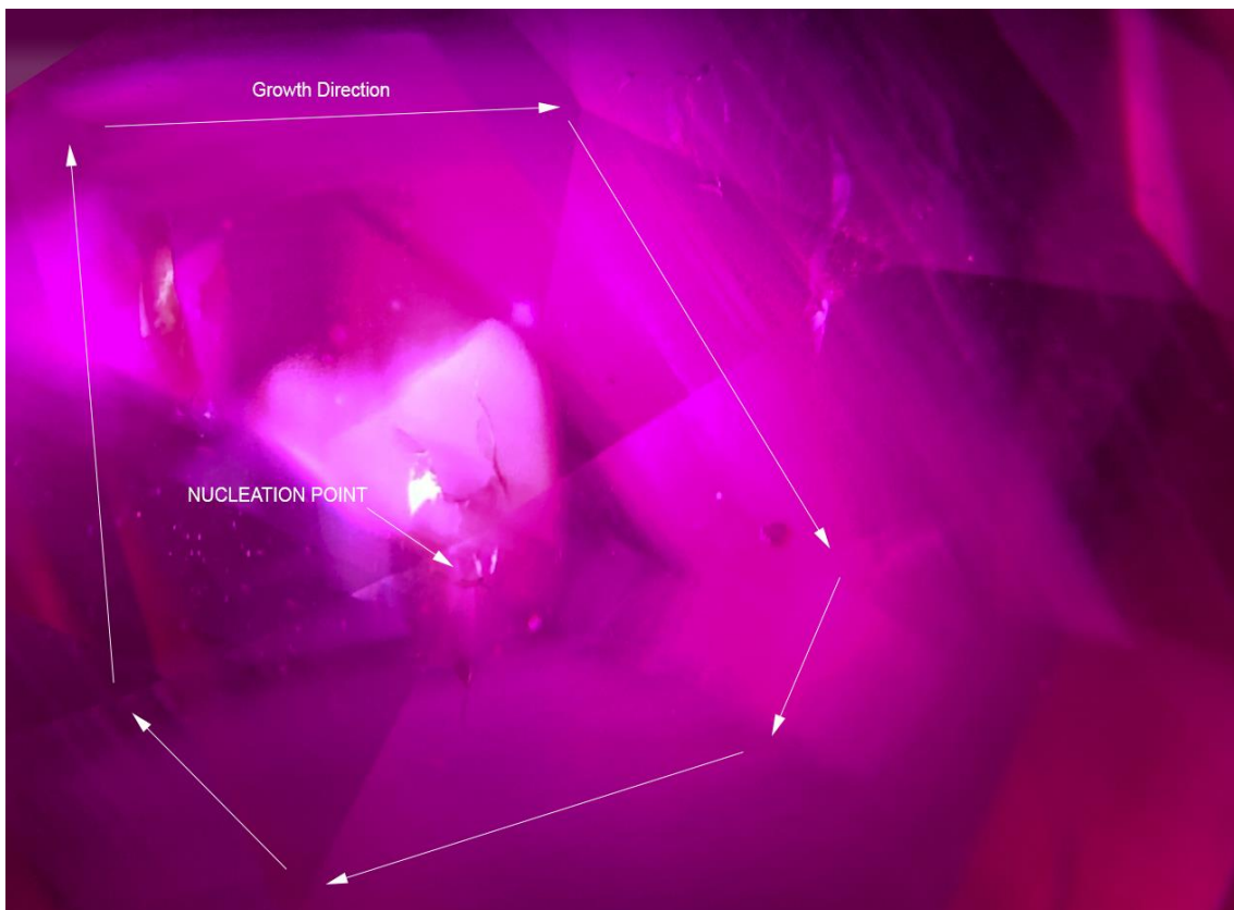
Nucleation point and growth direction of the Estrela de Fura, x90 magnification.
