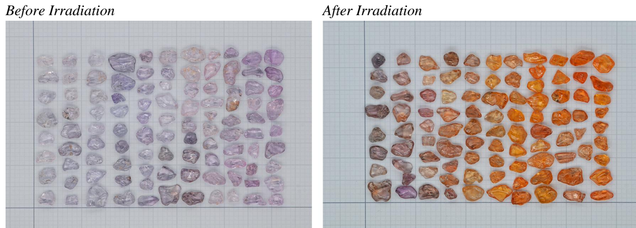
Figure 3: Gamma Irradiation of Pink sapphire before and after.
