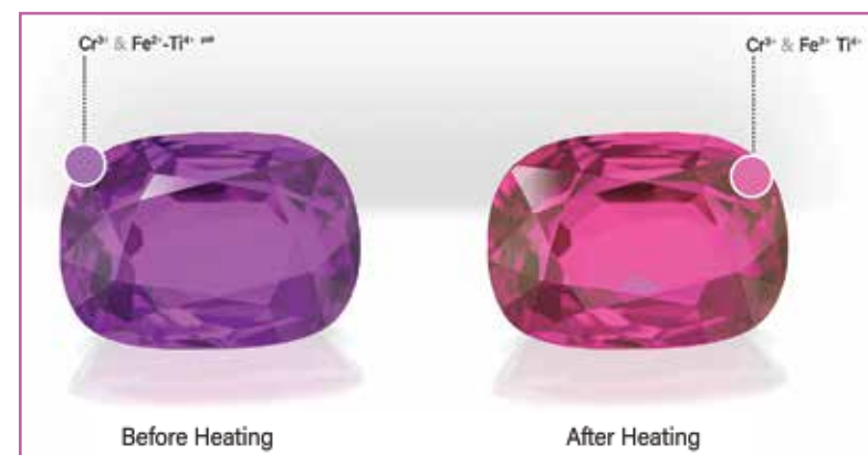
Figure 1. A 1.25 ct pink sapphire from Ilakaka, Madagascar before and after low-heat treatment. (Photo: M.P.H. Curti/Bellerophon Gemlab, reference collection No B76311)
